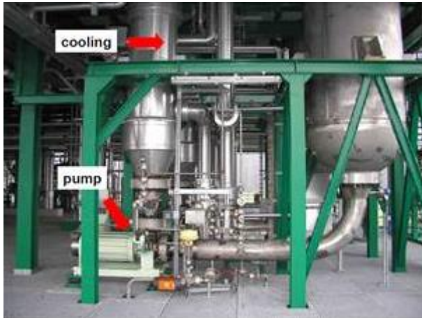
Bottom part of loop hydrogenation reactor
